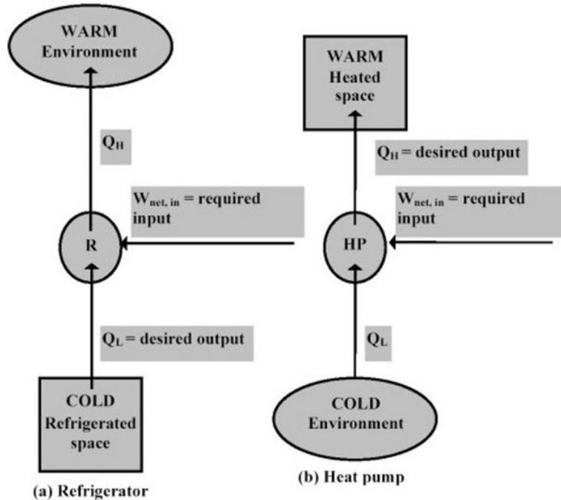
Figure 1. Refrigerator and heat pump working principle
