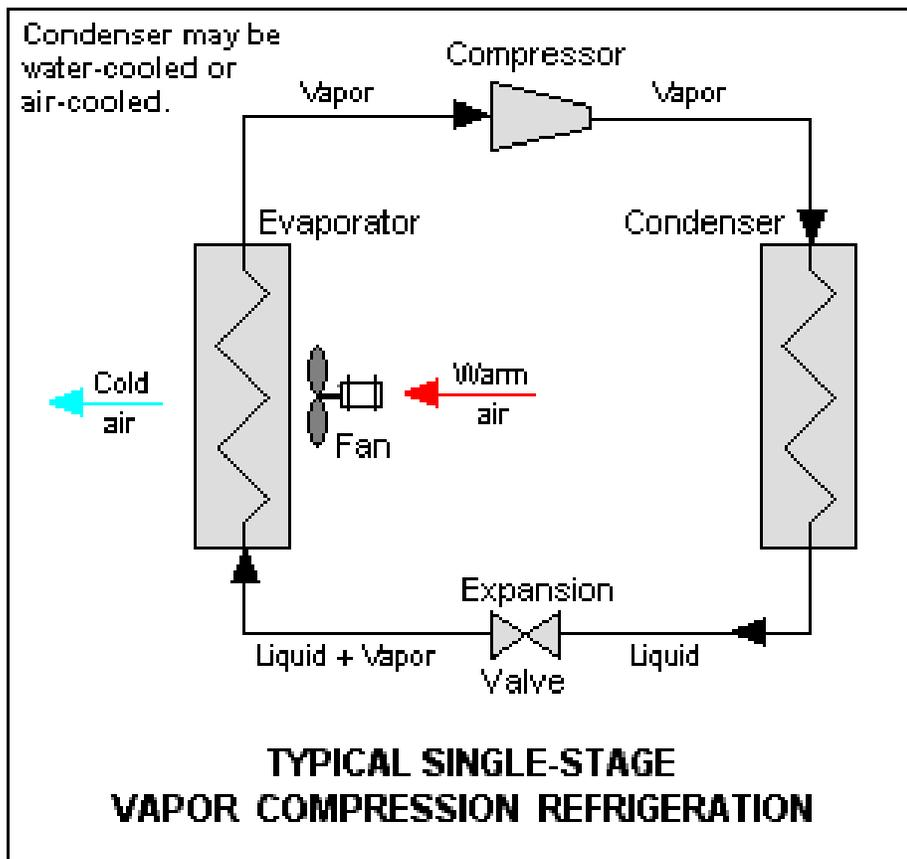
Figure 1. A schematic of A Basic Refrigeration System. Source: [http://en.wikipedia.org/wiki/Vapor-compression\\_refrigeration](http://en.wikipedia.org/wiki/Vapor-compression_refrigeration)
