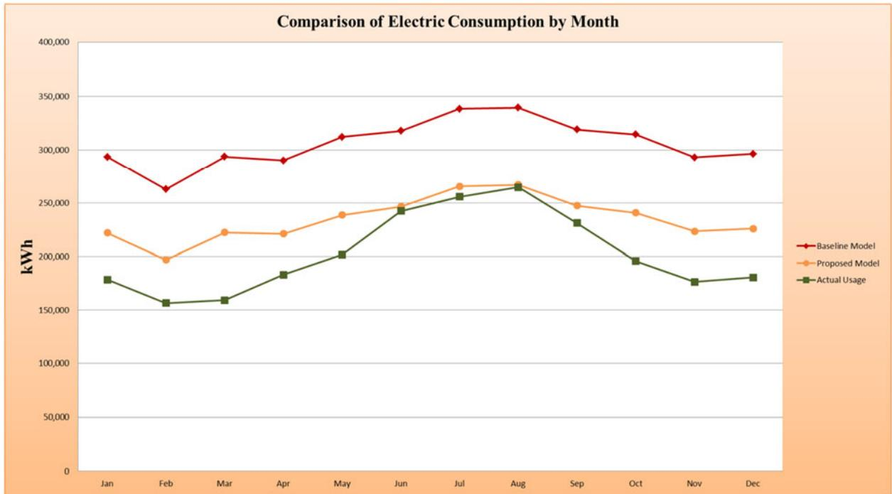
Figure 3. Comparison of electric energy use between simulation models and actual usage
